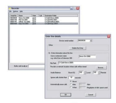
**BackOffice Digital Recorder** runs as a full-time utility recording all calls to and from every connected telephone. On those PBXs where caller ID is supported, it will also capture the caller ID and number dialed of every call and make part of the call record.
