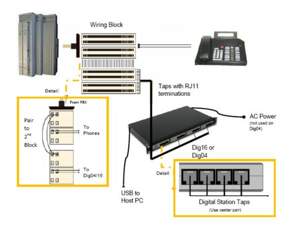
The Dig04/16 records directly off the Digital Station Pair of compatible PBX/Key systems using a parallel tap of the same pair that powers the Digital Phone. The above Diagram illustrates one way to accomplish the parallel tap required, although there are many ways to get to the same end.
