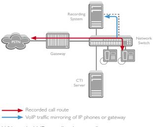
With passive VoIP recording the recording system connects to mirroring (SPAN) ports that reflect the traffic to be recorded
