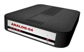
The Analog 02, 04 and Analog 08 Recorder hardware connect via a T-Connect Tap of an Analog Telephone Line or Analog Station. It derives power from the USB connection with the host PC.
