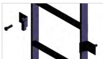
14. WALL BRACKETS Secures runway flat against the wall ICCMSLVWBK, 2 each
