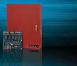
UL Listed 864 9th edition NAC Power Extenders are designed for hi-rise fire applications. Units provide 4 Class A or 4 Class B signaling circuit outputs. They range from 6.5 to 10 amps max. power output and are equipped with built-in sync protocols of all major notification devices.
