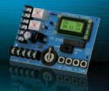
PT2724 Annual Event Timers are designed for a wide range of applications including home and building automation, security, access and lighting control, and more. With alphanumeric LCD display, built-in battery charger and EE prom memory – so you don't miss a beat (refer to page 122 for further info).
